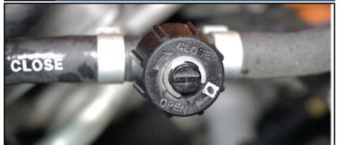
**B8. Cooling System Circuit: Coolant Discharge and Air Drain Procedure**
