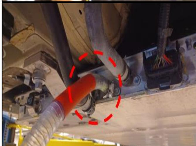
C17. **Cleaning the Cooling Circuit Section of Waste Heat Chiller**
